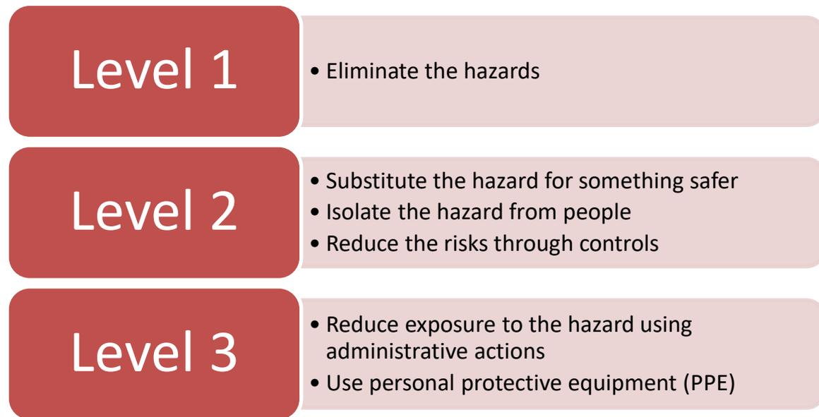
Level 1 controls are the most reliable and the most likely to provide protection. Level 3 controls are a last resort.
